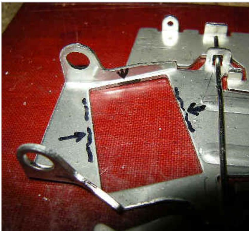
E2.3.7 JK X32 chassis for Super Production class: A small amount of material may be removed to facilitate installation of Wasp/Hornet Super Production motors as follows
